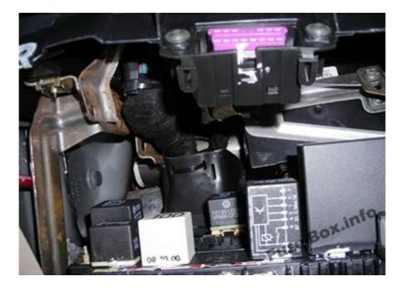
Additional fuses are available in the electronics module. The electronics module is located on the left side near the engine compartment partition.
