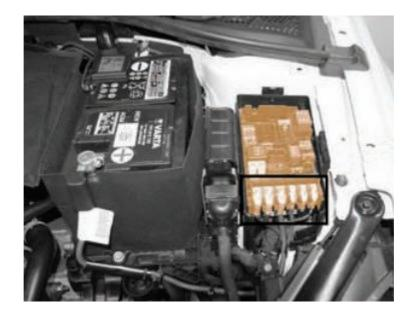
Consists of 2 sections: a communication section with fuses and relays, and a section for high power fuses.
