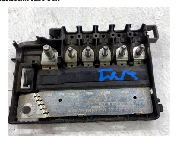
This power fuse box is installed in the cover on the battery.
